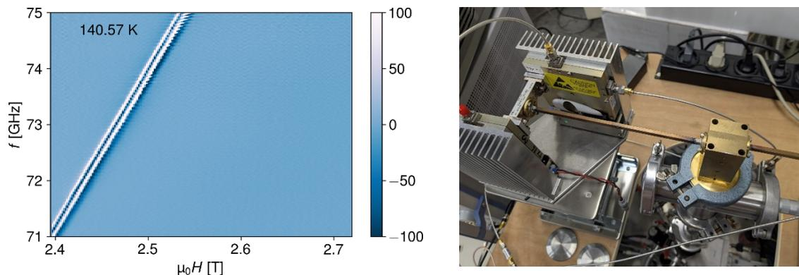
Figure 1: (left) Broadband VNA-FMR measurement of LPE grown YIG, at 140.5 K using the 70-80 GHz module. The raw data is processed by derivative divide. (right) 70-80 GHz and 80-90 GHz sending units, connected to the head of the sample insert on top of the cryostat. The connection is done with WR12 rectangular waveguides.
