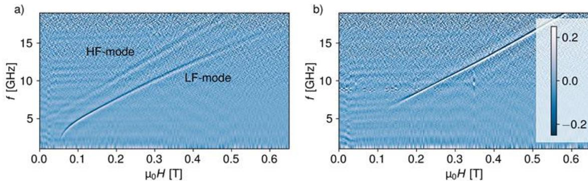
Figure 2: Broadband VNA-FMR measurement of the YIG 36 nm/ GdIG 30 nm/ Pt 4nm trilayer at a) 50 K and b) 200K. The raw data is processed by derivative divide and an FFT-filter. (Figure modified from [A]).
