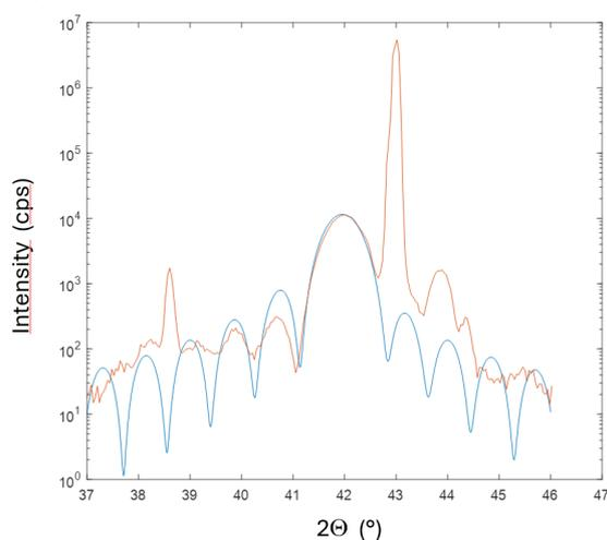
Figure 4:  $\Theta/2\Theta$  x-ray diffraction scan of a CoO film (11 nm) on MgO substrate (red line). The two sharp peaks are from  $K_{\alpha}$  and  $K_{\beta}$  diffraction at the substrate peak. A fit with a kinematic scattering model and strain relaxation away from the substrate is shown as a blue line.
